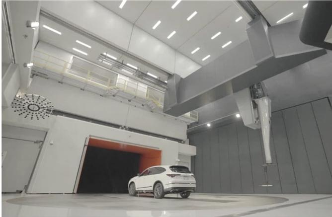
*Figure 5. The flow survey traverse positions a probe in the wake of a vehicle in the test section.*
