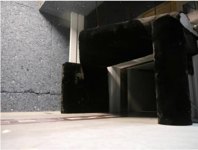
Figure 20. A model of the collector undergoing acoustic testing in the 1:8 scale model wind tunnel.
