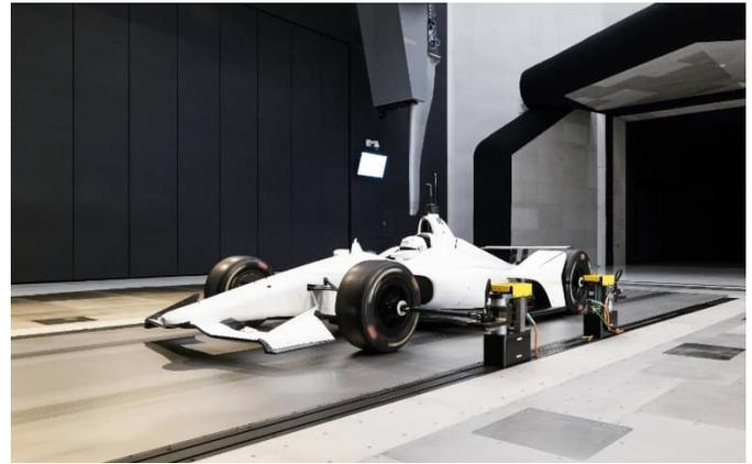
Figure 2. Motorsports testing up to 310 km/h is performed with the small nozzle and single belt moving ground plane.
