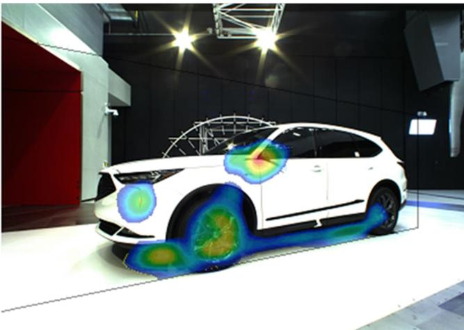
Figure 4. Broad-spectrum noise map image generated by the acoustic test system for a mass production SUV at yawed at 30 degrees with a 100 km/h wind.
