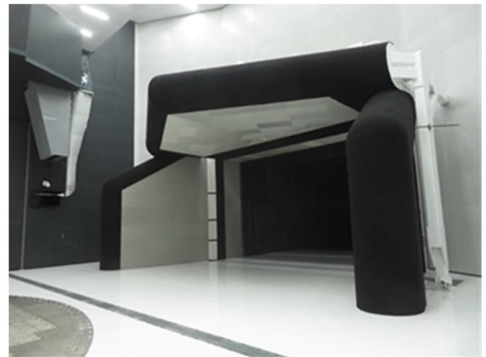
Figure 9. The collector in the HALO wind tunnel test section features swept leading edges covered with pile fabric.
