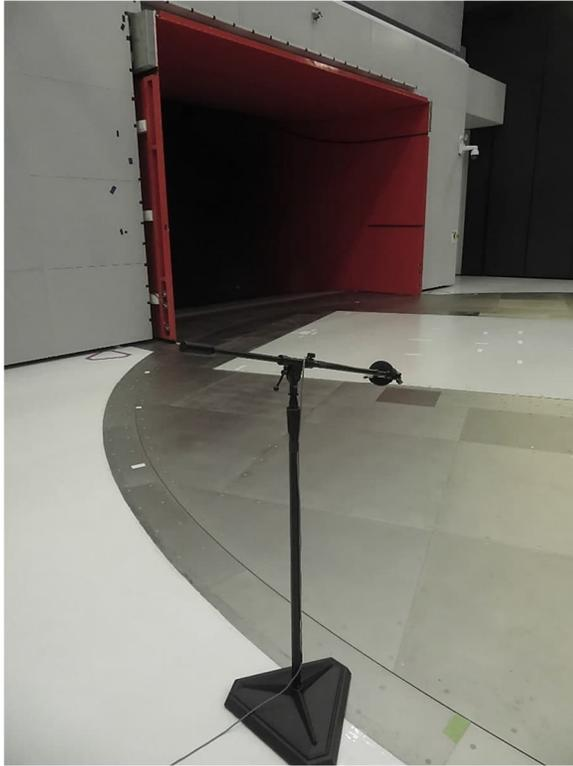
Figure 23. Microphone mounted on stand and positioned at (X, Y, Z) = (0, -6, 1) m relative to vehicle center. The MGP acoustic cover was installed, and the turntable was yawed when the photo was taken.
