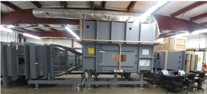
Figure 17. The 1:8 scale closed-return model wind tunnel during development testing.
