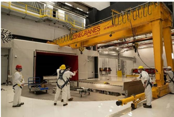
*Figure 6. Semi-gantry crane is used to transport MGP modules between the infield storage area and the turntable.*
