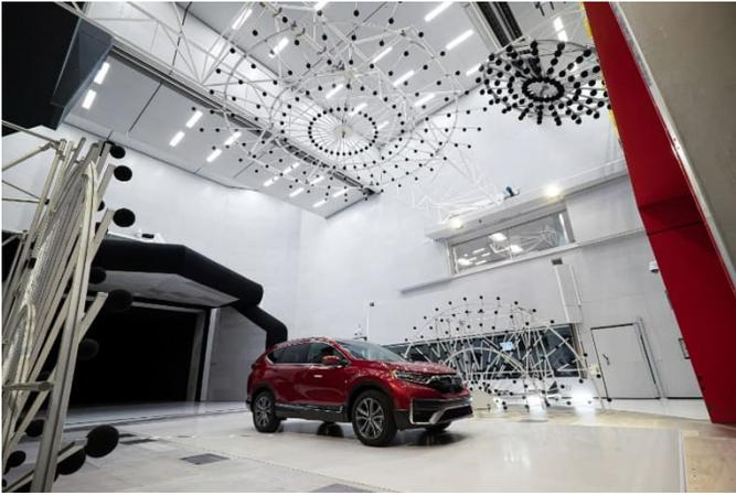
Figure 3. The test section configured for acoustic testing with exterior microphone arrays deployed.
